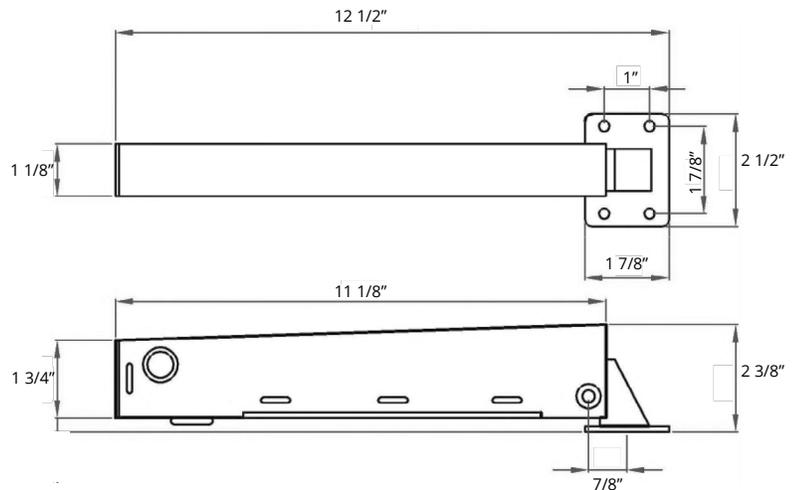
*The TB175 may not be compatible with offset hinge arrangements or arrangements that create more than 2" between gate post and gate, as it is critical to mount the closer as close as possible to the gate's pivot point.*
